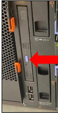
8. On the front of the POS blade, hit the clear KVM buttons for the monitor and keyboard and ensure both buttons are lit up.
