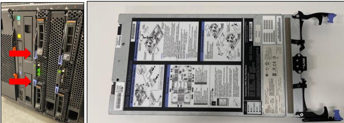
4. Extend the locking arm of the Management Module to unlock (orange handle) and pull out and set aside.
