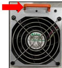
7. Extend the locking arm of the Power Supply Module to unlock (orange handle) and pull out and set aside.
