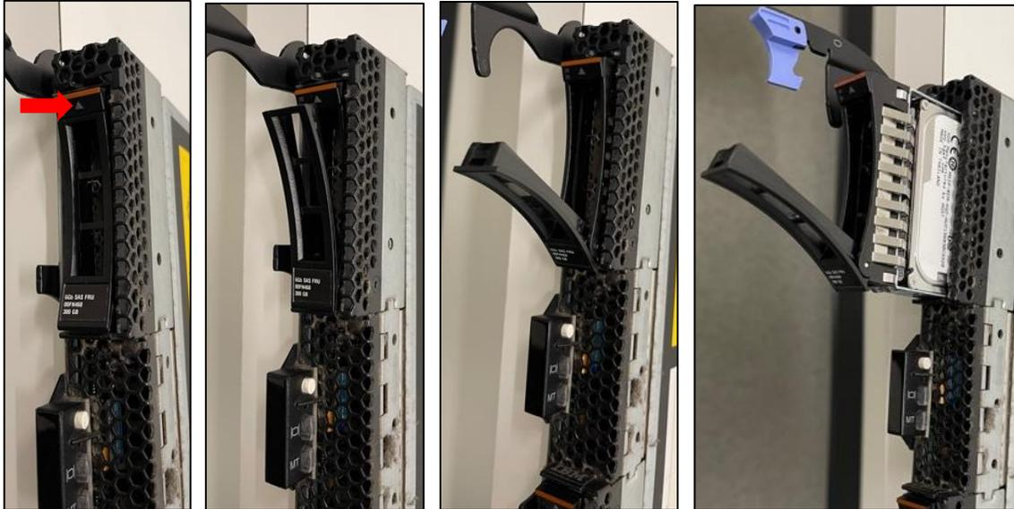
3. Extend both locking arms to unlock the blade from the chassis (purple handle)
