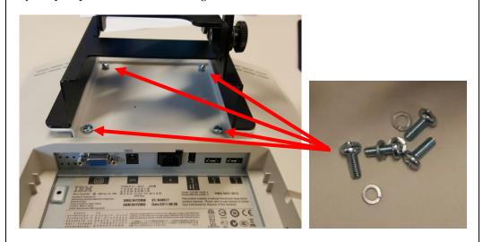
7.12 Carefully mount the monitor and swing arm back onto the Uniweb wall. Tighten thumb screws to secure in place.
