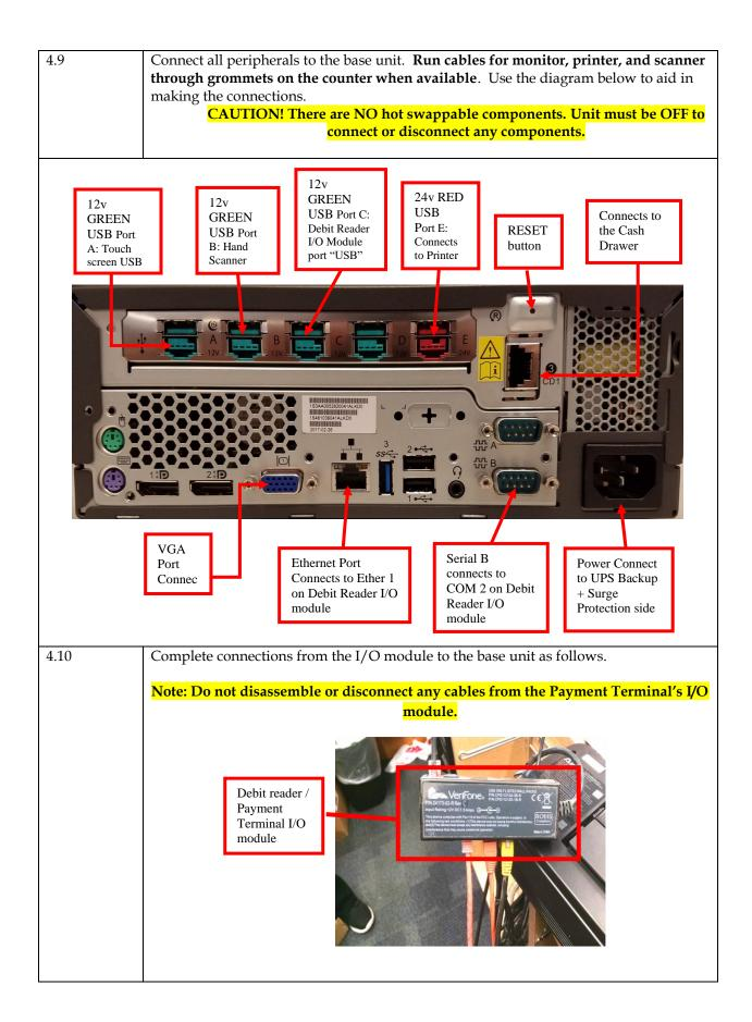
Connect cables **FROM** the I/O module **TO** the register base unit.
