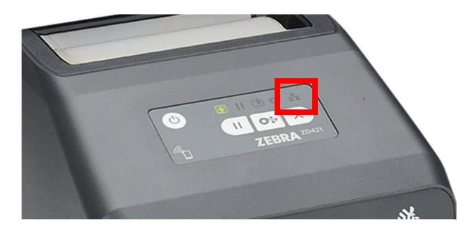
3. Hold down the Feed and Cancel buttons (the middle and right button) for approximately 3 seconds to print out the configuration sheets.
