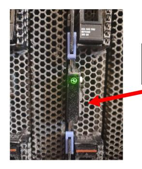
KVM Switch buttons are located under white power button.
