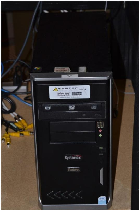
Video system is a PC based system utilizing either analog video capture cards, IP connected cameras or a combination of both.
