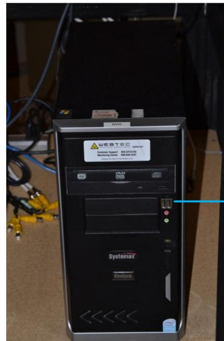
Standard Serial to USB adapter terminating wire from Eagle system and plugged into open USB port on DVR
