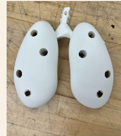
PLA filament printed 3D models, designed for adequate space & airflow for the sensors. The holes allow for ventilation and wiring.
