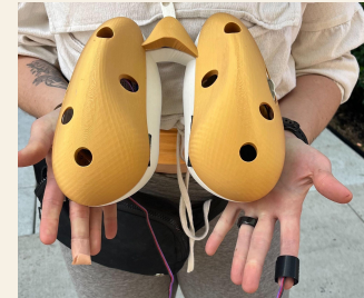
PLA filament printed 3D models, designed for adequate space & airflow for the sensors. The holes allow for ventilation and wiring.
