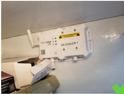
Figure 3.4a- Correct RX Cooler Install
