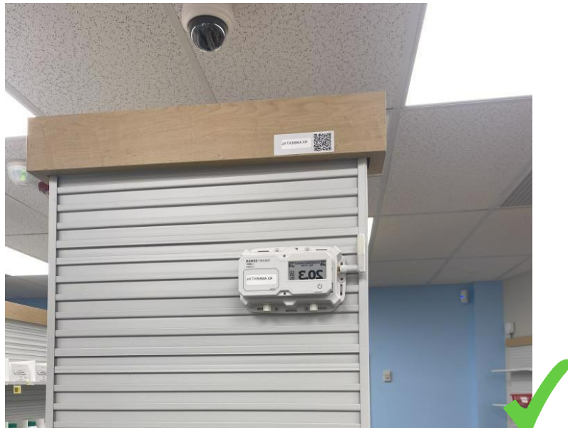
Figure 4.1- Proper RX Ambient Placement
