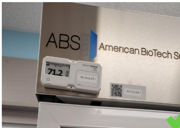
Figure 3.5a- Correct QR & ZSensor Placement for RX
