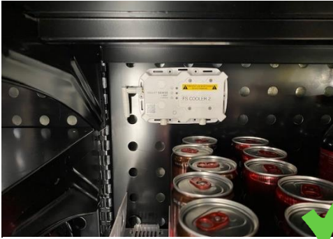
Figure 2.2a- Correct FS Node Positioning
