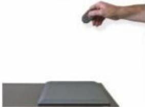
2. Lower tester towards deactivator pad until tester visually and audibly alarms. This indicates that the RF deactivator is functioning properly.
