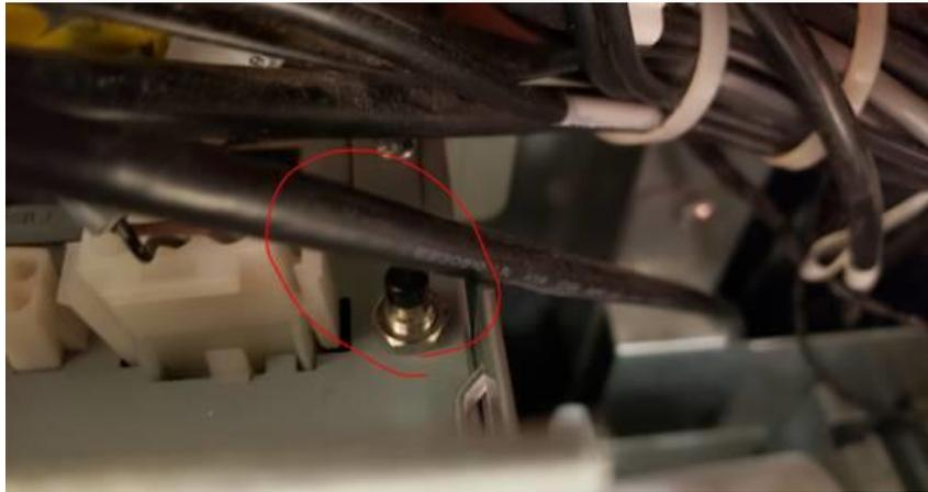
6. Turn off SCO by pressing and holding power button for 3 seconds **OR LESS** (If you release too quickly the register will reboot). The power button is located on front right corner of the processor (refer to above images). Register will start to shut down and will display shutdown on display.
