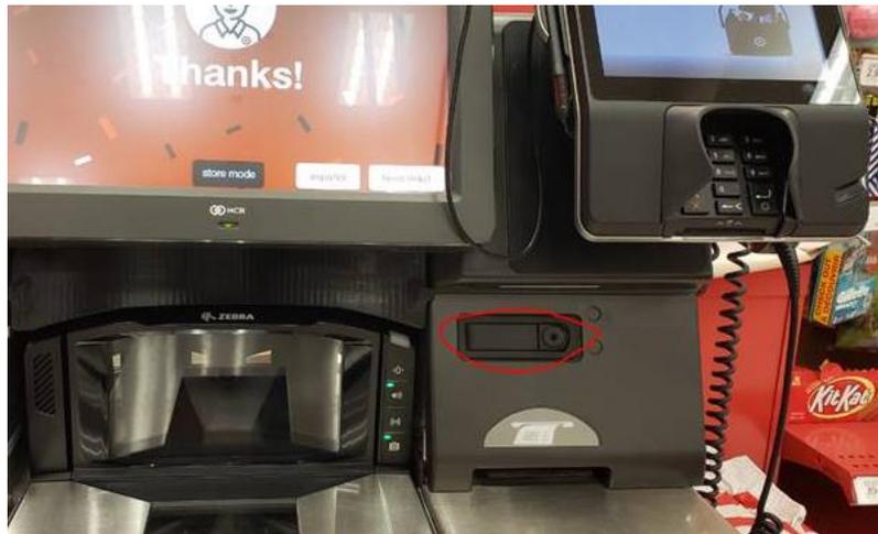
5. Open front cover by pressing on the lock on right side of SCO and lifting cover up, shown above.
