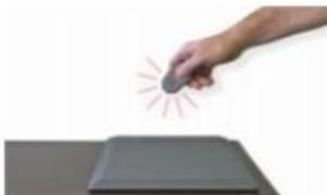
3. When the tester is removed from deactivator field, the tester will automatically stop alarming. Release the tester button to make it inactive.
