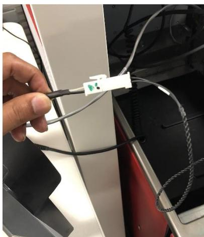
14. Plug in EAS cable. Attach the male cable from the new scanner and female cable from existing register as shown in the image above.
