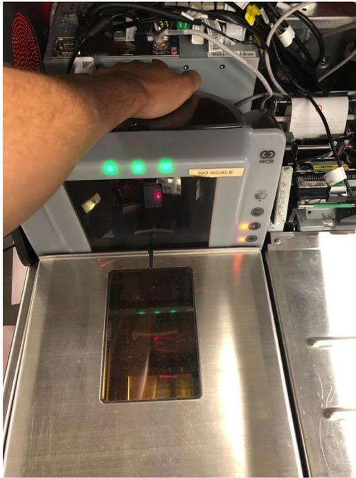
7. Remove old flatbed by lifting unit out of well (shown in the image above), set aside, unplug the 3 cables from the back of the flatbed scanner:
