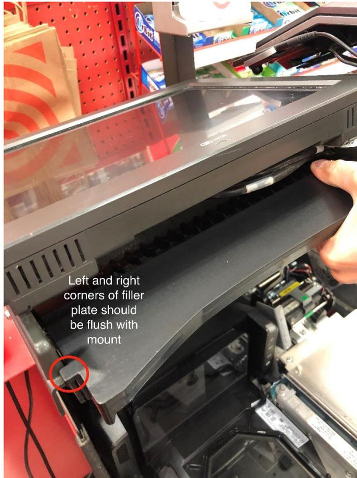
16. Take out the filler plate, make sure it fits, and verify the surface behind the monitor is **dry**. Take off the seal and make sure the sticky side is facing you. Using both hands, attach the sticky side of the filler plate onto the surface behind the monitor and hold for at least 10 seconds.
