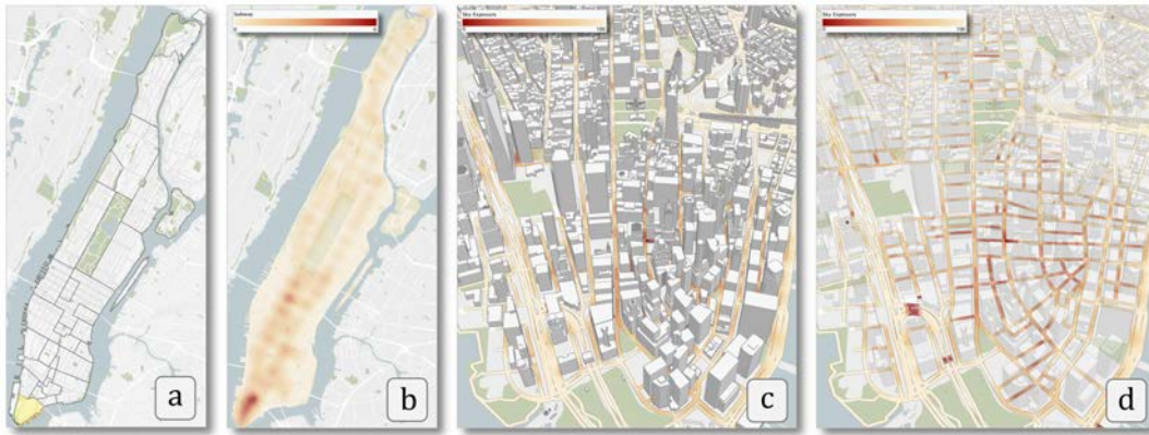
Figure 4: Examples of visualizations of different data layers supported in Urbane. (a) Polygon layer showing the different neighborhoods in Manhattan. The polygon corresponding to the Financial District is highlighted (yellow). (b) A grid layer representing the density of subway stations in Manhattan. (c) Representation of 2D and 3D data layers of the city in a single view. The heat-map along the road network represents the sky exposure along those streets. (d) Transparency can be used to avoid occlusion of the 2D layers by the 3D building geometries.
