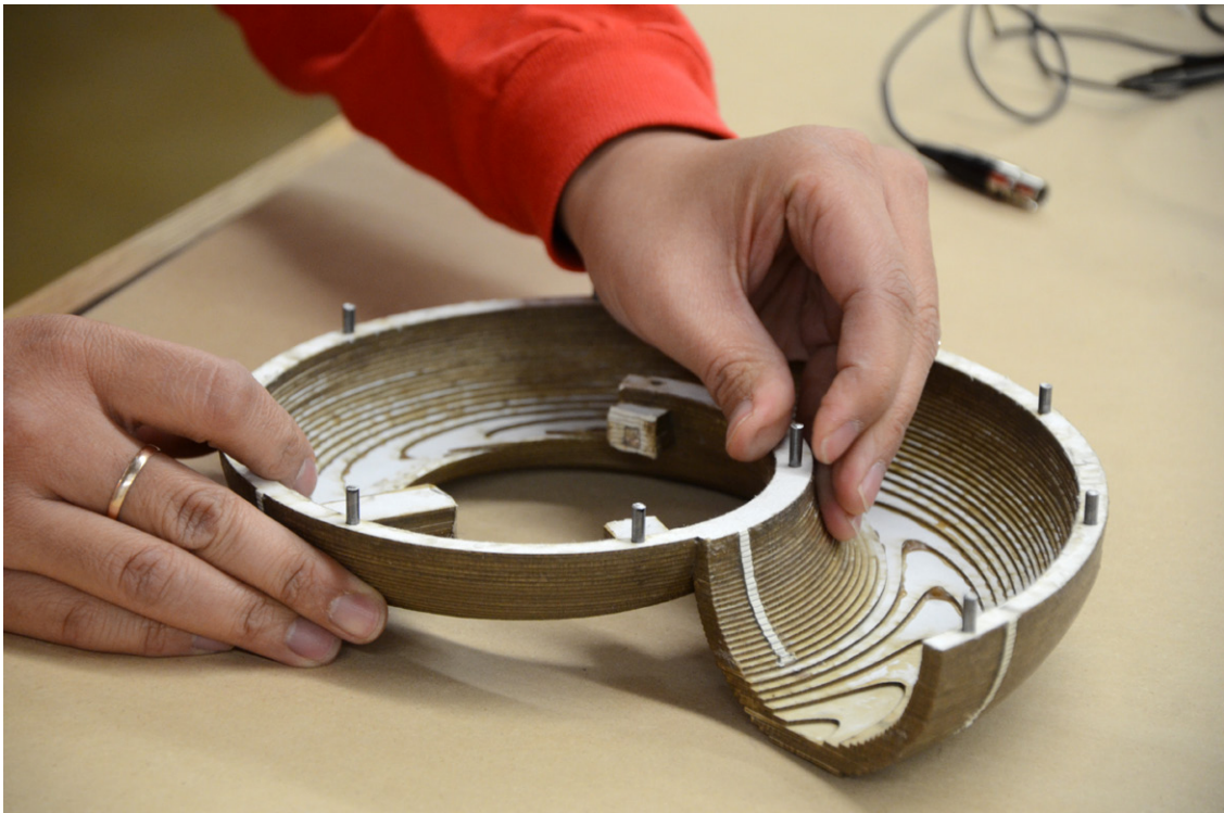
Installing guide pins for the body.
