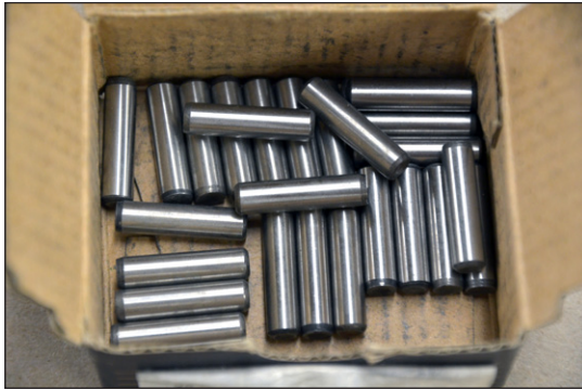
1/4" precision ground steel dowel pins.
