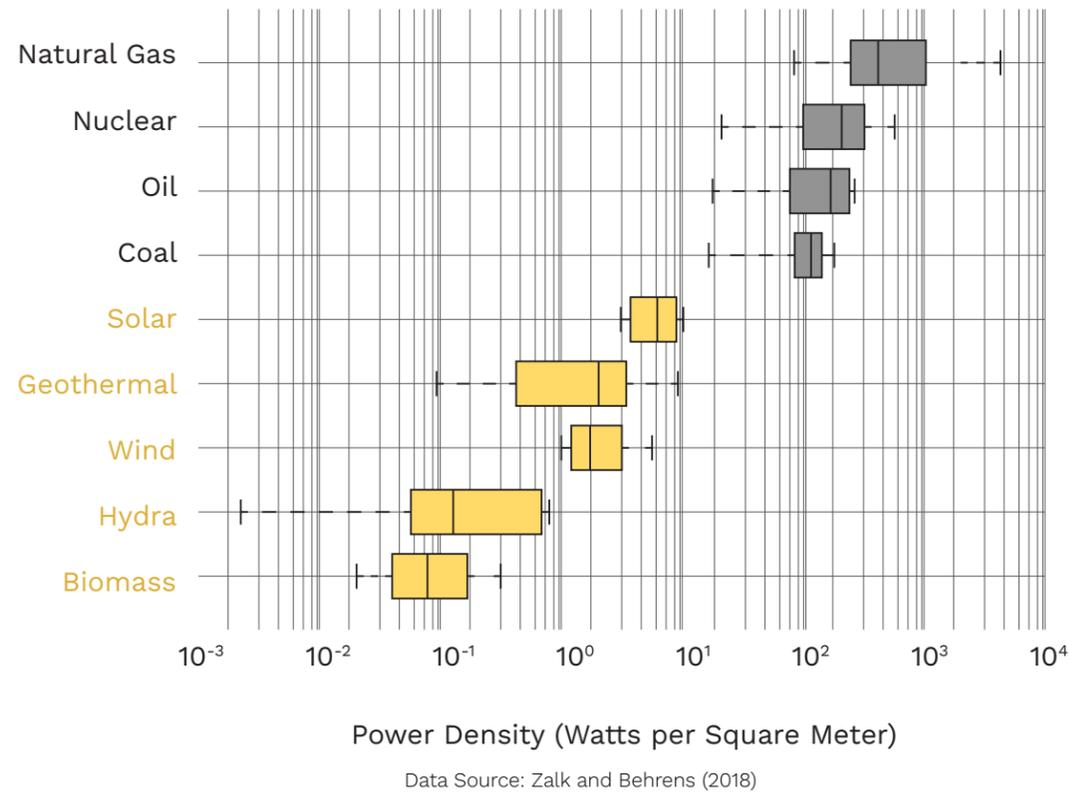
The concept of power density is important in evaluating the feasibility of replacing peaker plants. Power density is measured as output capacity per unit area and, generally, solar panels have a substantially lower power density than that of natural gas turbines, like those located at the peaker plant sites.
