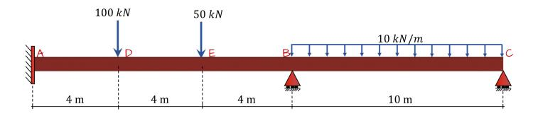
Q. Determine the support reactions, shear force diagram and bending moment diagram for the structure shown above.
