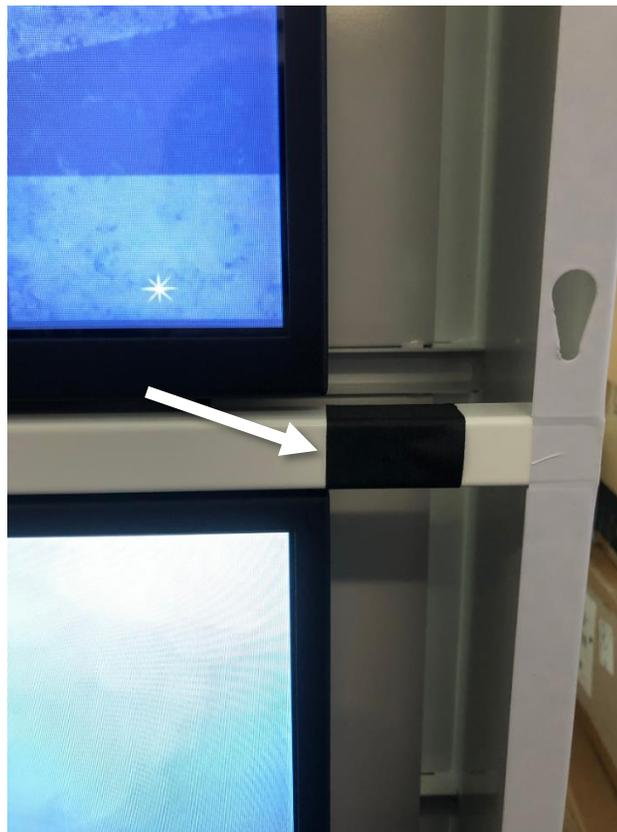
5. Pull release cords for both monitor mounts to unlatch. Release cords are located behind the display speaker just above the DMP. Extend monitors forward, being very careful not to put any strain on the cables behind the monitors.
