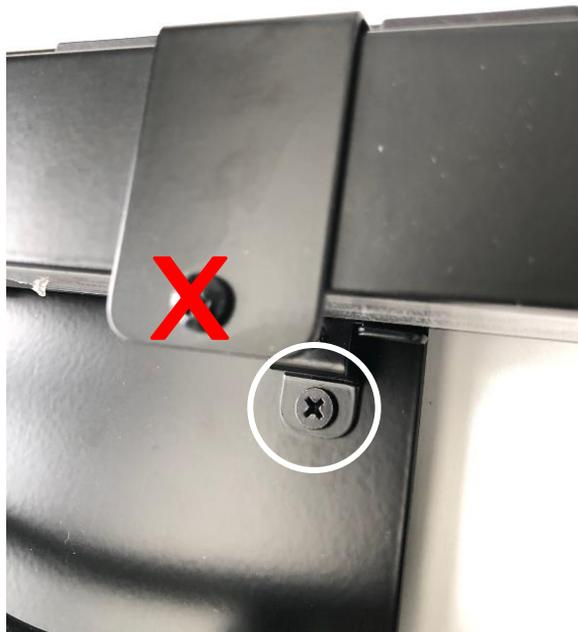
7. If present, remove and dispose of AX6959 DMP security cover by unscrewing the 2 silver thumb screws on the right side.
