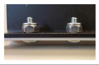
7.11 Lay adapter plate on monitor and tighten screws and washer onto monitor.
