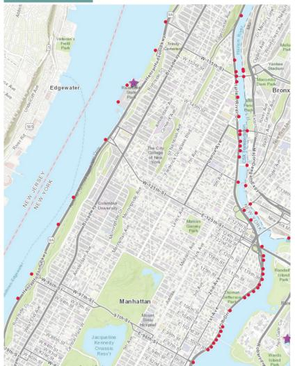
The storm water and sewer infrastructure of Harlem is less well-equipped to handle flooding events without depending on sewer outfalls into, primarily, the Harlem and East Rivers. Thus, raw sewage and storm water are dumped directly into the rivers rather than diverted to treatment facilities.
