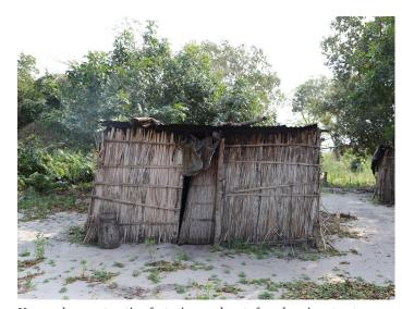
$\label{lem:vertex} \textit{Vernacular construction featuring reed mats for a housing structure} \\ \textit{used for cooking}$
