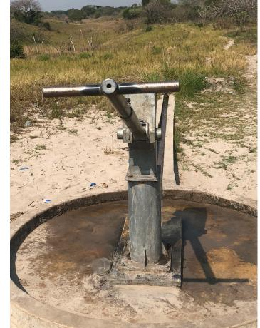
Manual hand pump for irrigation well
