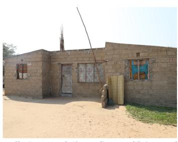
$Local\ housing\ constructed\ with\ cement\ (limestone\ and\ clay),\ water,\ and\ sand\ from\ rivers$
