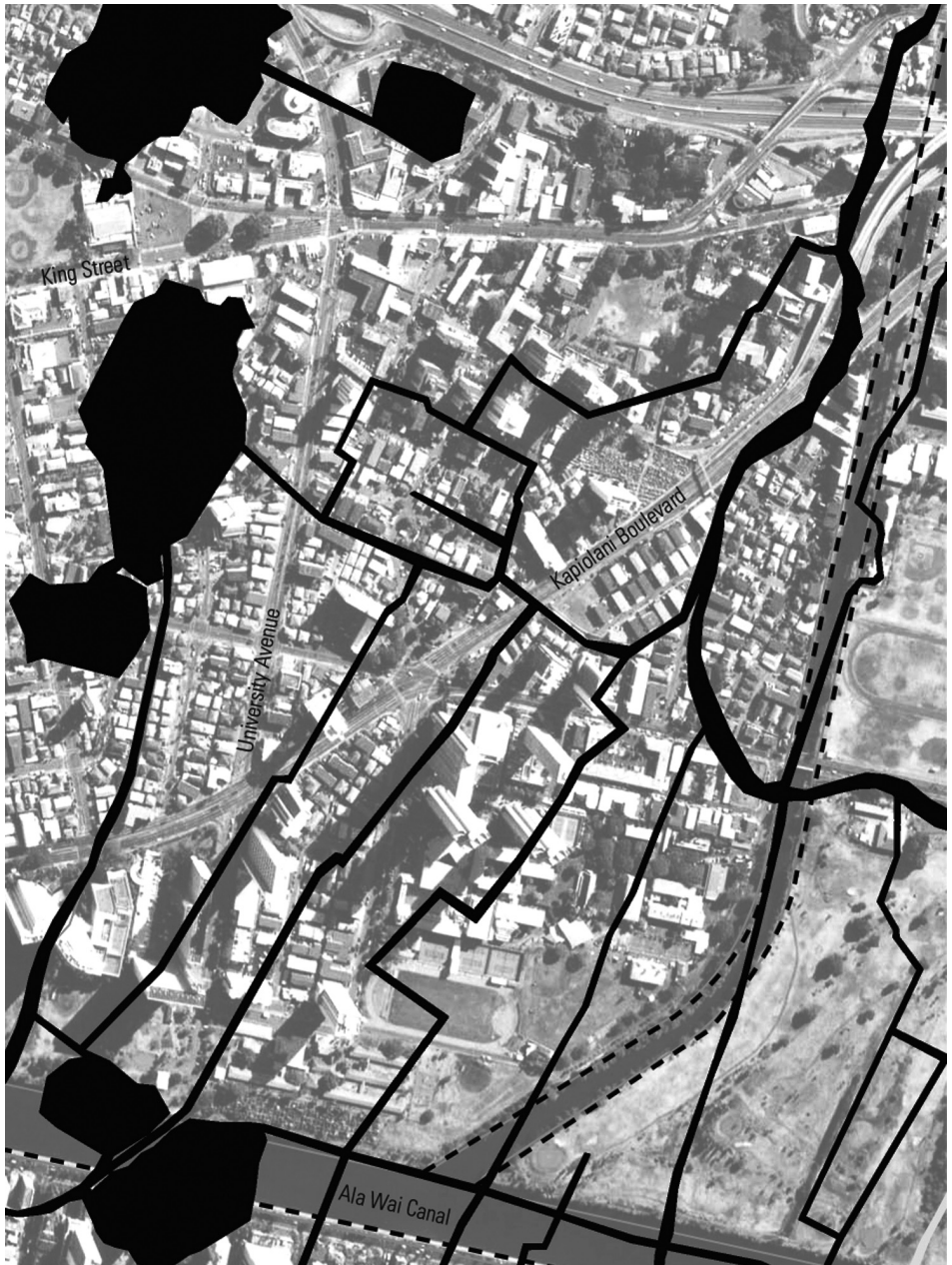
Figure 1. This image shows a USGS aerial photo of Mō'ili'ili overlaid with the traditional 'auwai system, in black. The solid patches to the left indicate ponds, while the thick band to the right is the original stream, which is now channelized (dashed line)
