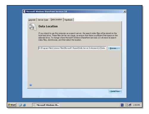
The Data Location tab allows you to specify where the WSS v3 program files will be stored. By default these will be installed in c:\program files\common files\Microsoft shared\web server extensions\12\data. You can specify any location by changing the entry displayed. It is recommended that you only change the drive letter if necessary to ensure compatibility and ease of future support.
