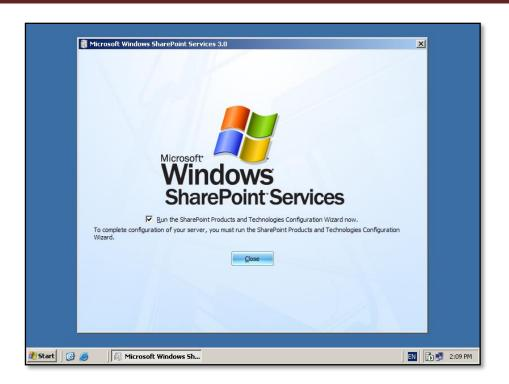
When the installation is successfully completed you will see the above window. By default, the *Run the SharePoint Products and Technologies Configuration Wizard now* option is selected. If you wish to configure WSS v3 at a later stage simply uncheck this option. Press the **Close** button to continue.
