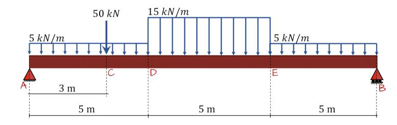
Determine the bending moment and shear force diagram for the structure shown above.
