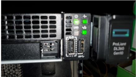
Call the ROC and inform them that the keyboard and monitor are attached to the New Gen10 server and you are ready to begin the Back end process. The ROC will Flag the server for Back end and provide you with the username and password to begin the process.
