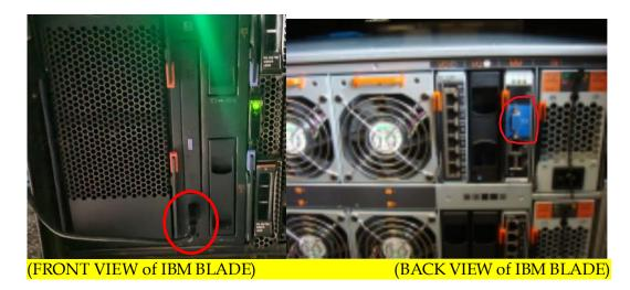
Connect Keyboard to FRONT and monitor to BACK VGA port of blade chassis.
