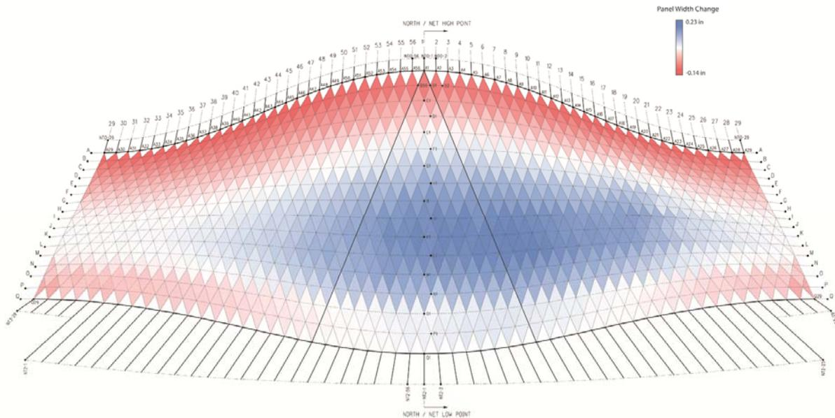
Fig. 11. Assessment of changes to panel shape due to environmental movements. One of 815 load cases shown.
