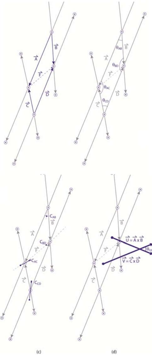
Fig. 5. Mathematical model of cable net geometry.
