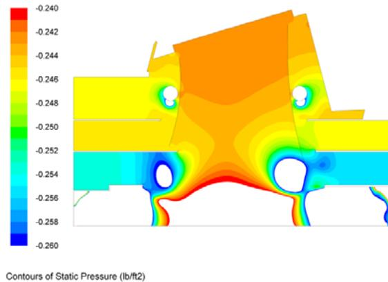
Fig. 8. A computational fluid dynamic (CFD) model was generated to determine air pressure incident on each panel.
