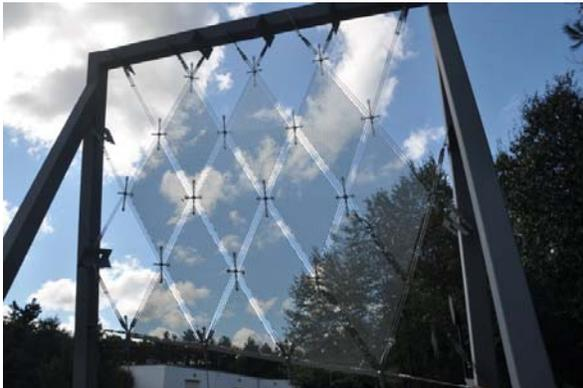
Fig 13. A full-scale mock-up of a 13-panel portion of the net was prepared by the contractor in accordance with project specifications.
