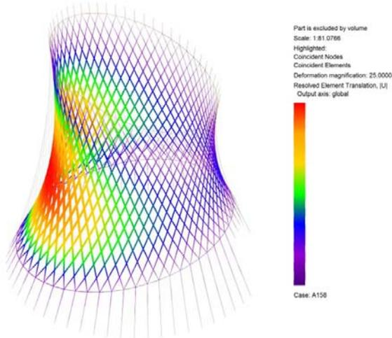
Fig. 9. Cable net deformations caused by environmental loading. (One of the 815 load cases studied.)
