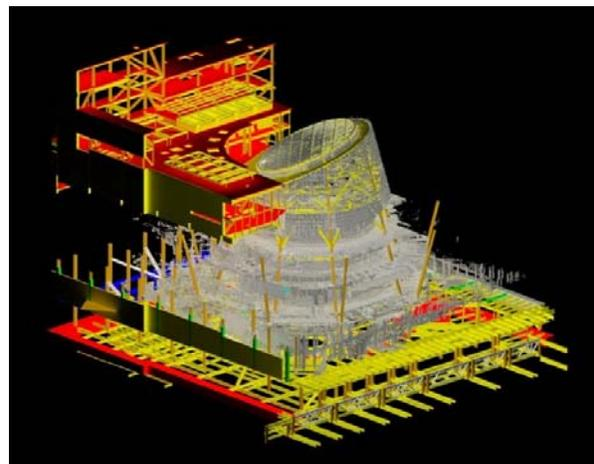
Fig 14. LIDAR survey data (shown in grey) overlaid on the project BIM model.
