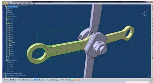
Fig. 10. Parametric definition of horizontal armature
