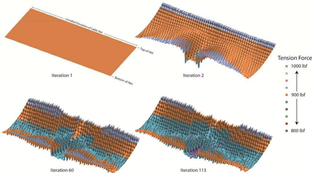
Fig. 4. Iterative development of prestress distribution forces.
