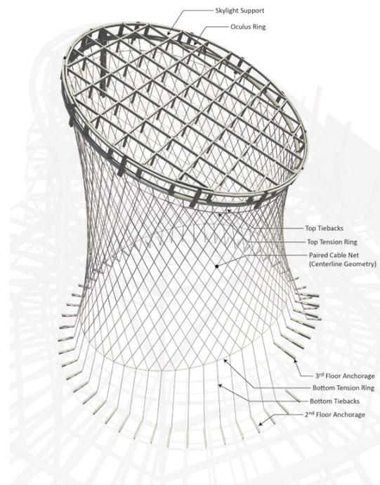
Fig. 2. Cable net components and boundary support.
