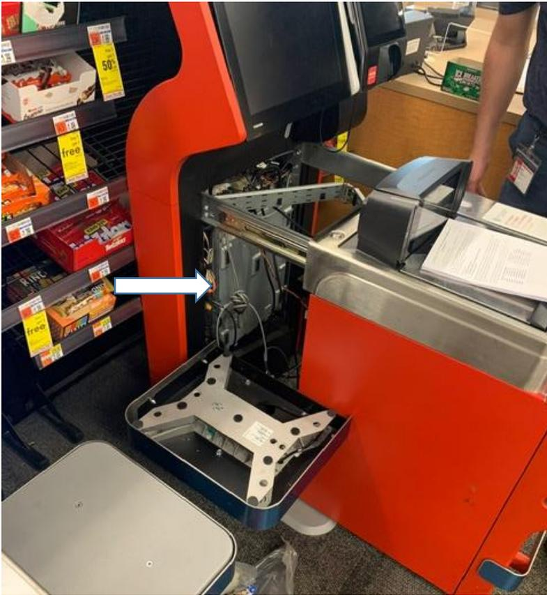
You would only have to remove the top of the shelf if it is bolted to the base
