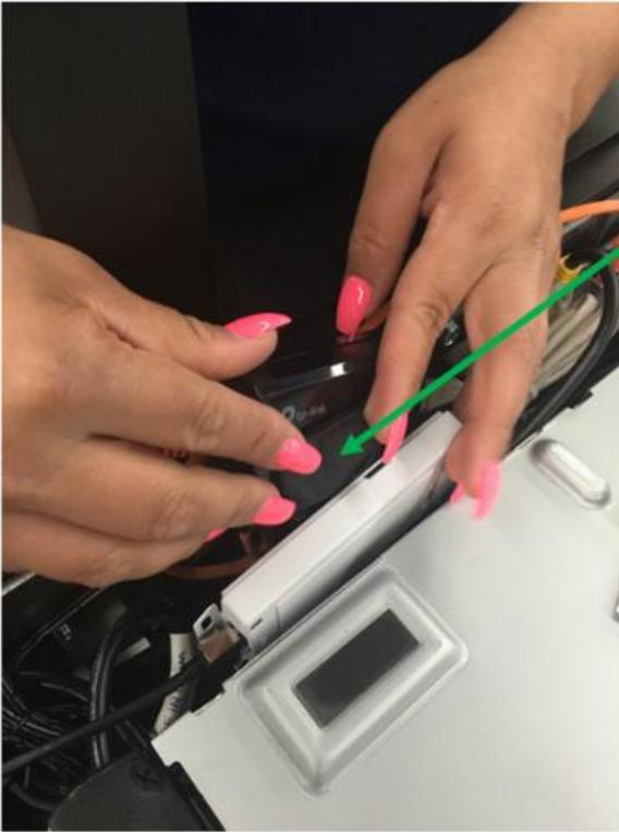
Install an adhesive backed Velcro between the Axis Main Unit and the Tp-PoE Injector Power Unit
