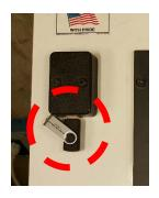
Plug your USB stick into the port on the top-left of the control panel.
