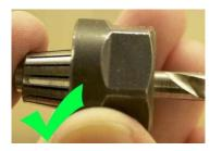
Once assembled, place the tool back into the mill and finger-tighten the nut onto the spindle. It should look like this once it's in place. Then use the wrenches and give only 1 quarter turn to tighten it.
