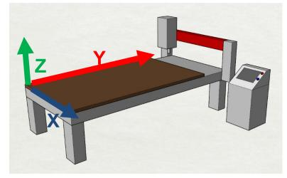
While still in the **JOG** screen, use the **XYZ** control pad on the bottom-left of the control panel to move the gantry and head around manually.
