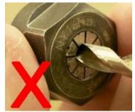
The collet should not compress around any portion of the endmill's cutting blade.
