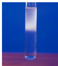
Fig 10. Test Tube Showing a Positive Emulsion Test for Lipids.
