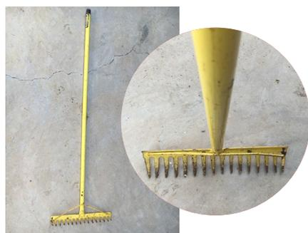
In the creation of your vegetable garden you will need a sturdy tooth rake as opposed to the more flimsy 'leaf rake'. A leaf rake is designed to rake up leaves. But we need a tooth rake to flatten our planting beds and remove large stones and old roots from the soil.
