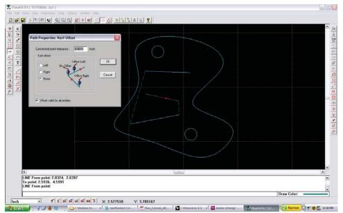
This creates the beginning of the path and the read arrows indicate the direction and orientation of the jet as it travels.
