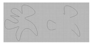
The closed shape on the left will cut in approx. half the time required to cut the open shapes on the right because of the time required to start and stop the machine at the endpoints.
