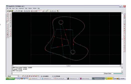
If there are more parts to path you can continue this process alternating between manual and automatic pathing as necessary.
