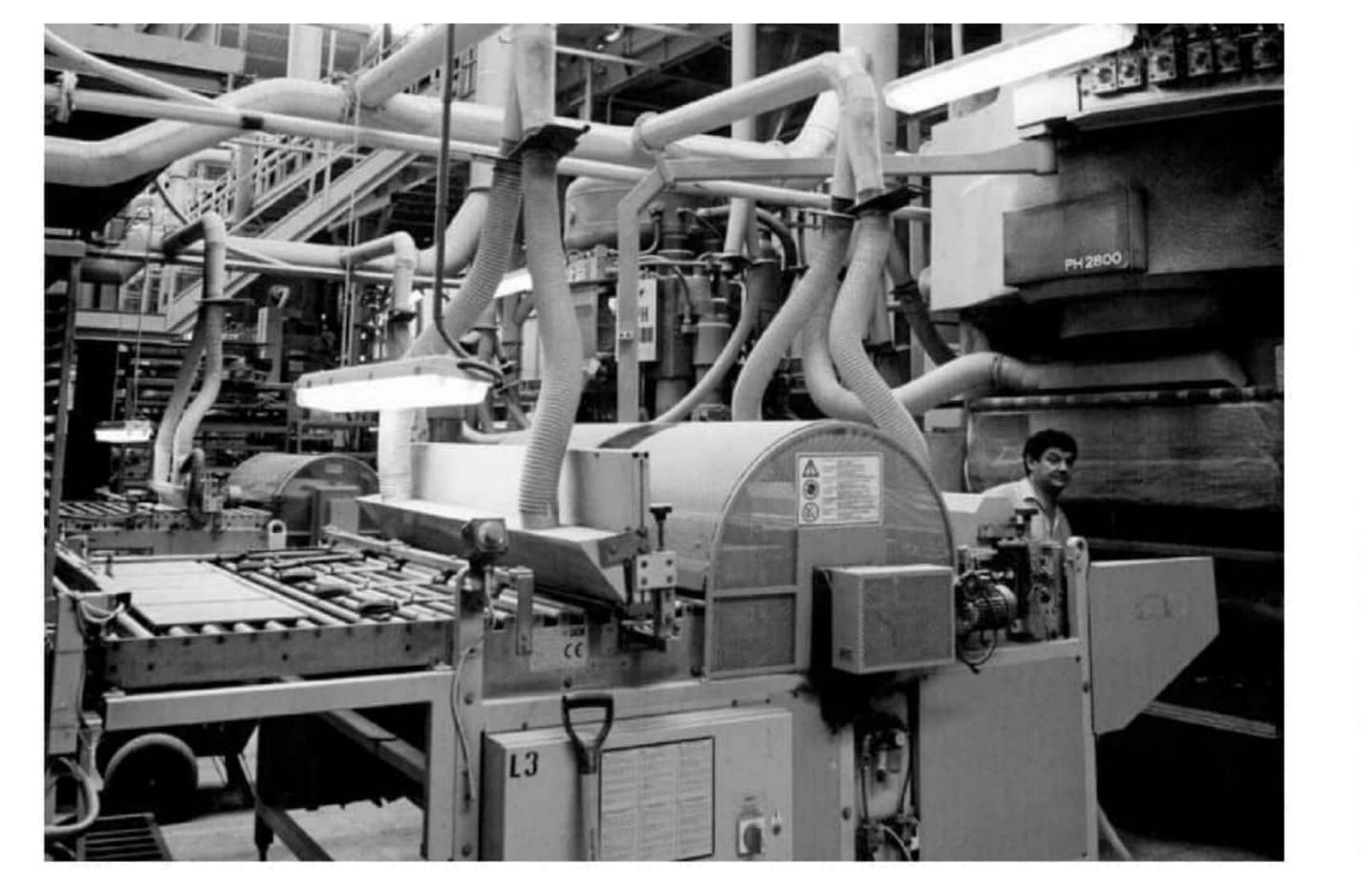
4. Forming - Most common method is dry pressing. Material is compressed, where steel plungers apply pressures of up to 2,500 tons of the powder
