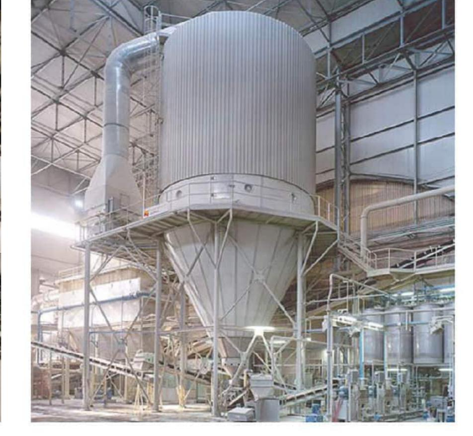
3. Spray Drying - Process of removing excess water. This is done by pumping the slurry into an atomizer, turning the mix into a powder which is ideal for forming.
