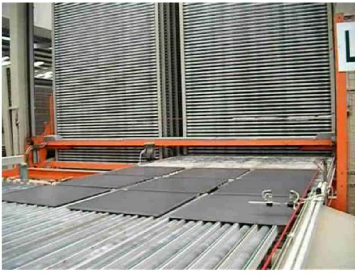
5. **Drying** - After forming, ceramic tiles need to be dried in an environment with high humidity. If the ceramic tiles were made with the wet method, humidity levels would need to be higher. This process of creating ceramic tiles can take several
