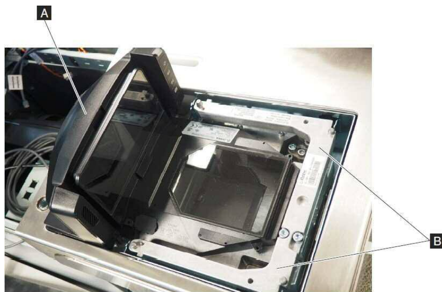
Figure 195. Scanner/scale lift points
