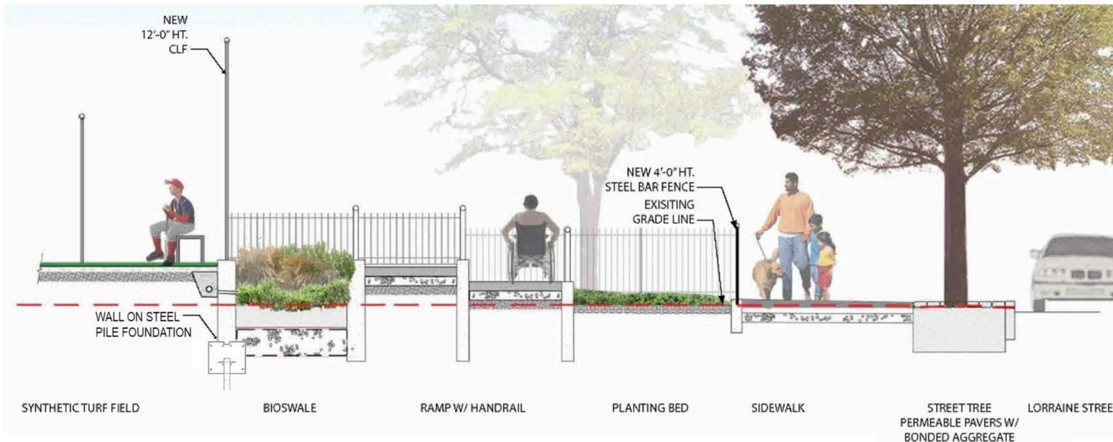
The lead-contaminated soil in the Red Hook Recreation Area ballfields will be capped by a demarcation layer, clean fill, a drainage layer, and synthetic turf while being enclosed by a retaining wall
