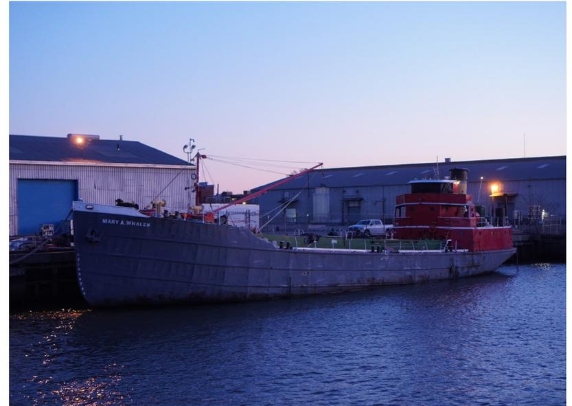
The Mary A. Whalen ship, from which PortSide NewYork operates, is listed on the National Register as a rare surviving example of a bell boat -- a ship controlled from the engine room by telegraph signals
