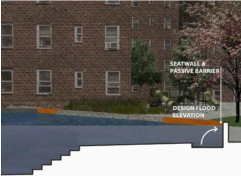
Rendering of NYCHA and KPF's "lily pad" design during flood conditions. A raised courtyard, combined with a deployable flood barrier, would allow water to pool without entering the Red Hook Houses
