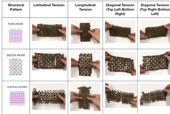
**Figure 3: Results of Performance Analysis through Fabric Handle.**
