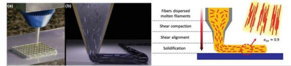
Figure 1: Orientation of fibers within an ink (Source: Compton and Lewis, 2014); High degree of material orientation in the printing direction (Source: Yu et al., 2021)
