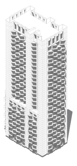
The living rooms of each unit would include a balcony. This balcony is the changing parameter within our design process. The protrusion of the balcony is adjusted according to how much sunlight each space captures.
