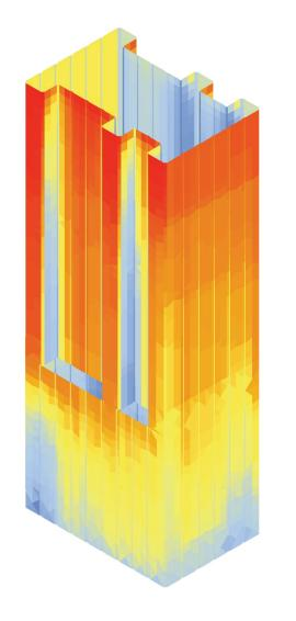
The upper floors of the facade capture most of the sunlight. In this diagram, red represents the most time exposed to the sun. While blue represents the least amount of time exposed to sun.
