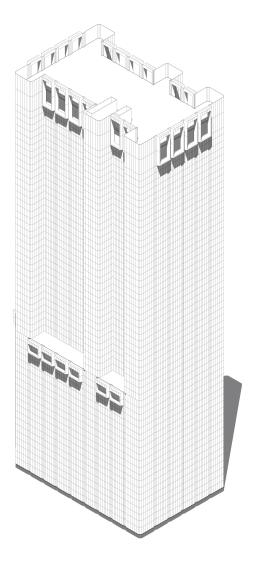
The façade at 33 Thomas Street, formerly known as the AT&T Long Lines Building, reflects the original use of the building. The windowless skyscraper was used for telephone exchange. The façade is made of precast concrete panels clad with granite.
