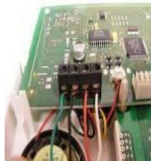
TERMINAL CONNECTORS OF THE 6160 KEYPAD
