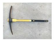
A pick is a heavy hand tool that is used to break up hard ground by swinging it over head and driving the hard metal point into the ground. The head is usually slightly curved and ends in a sharp point.
