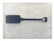
In the garden we typically make use of a flat edged spade, rather than a shovel which has more of a curved blade. The space is used for digging pathways in the garden and moving soil as well as removing weeds and rubble.
