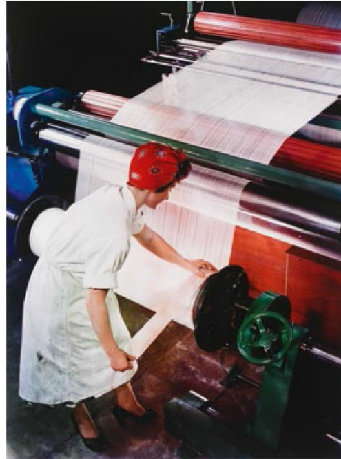
Maurice Broomfield, Preparing a Warp from Nylon Yarn, British Nylon Spinners, Pontypool, Wales, 1964 © Estate of Maurice Broomfield
