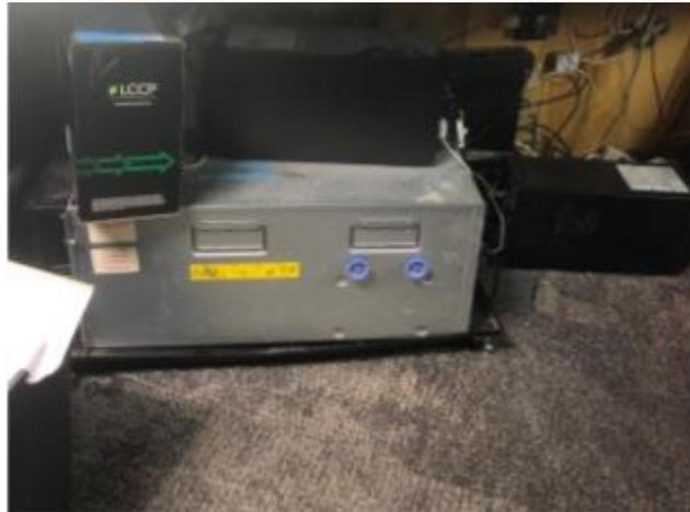
Remove the cover from the front of the blade chassis. Pull down slides located on the top left and right of cover and remove. This will expose the three blade units.
