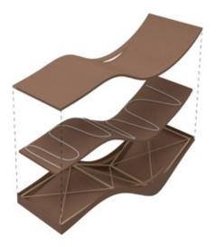
Figure (7): Axonometric diagram showing skeleton, first layer, heating wires, and exterior layer
